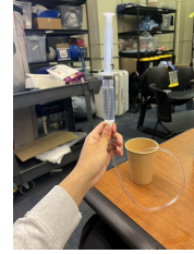
Figure 3: Filling syringe and tubing with water
