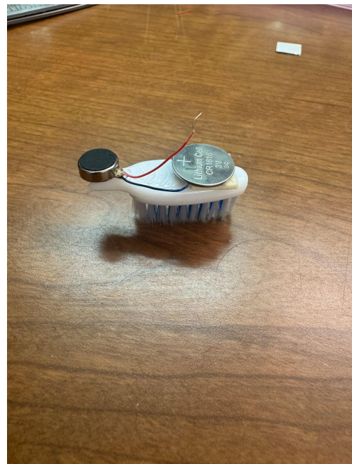
Figure 8: 3V cell battery is placed on top of the blue wire. The back side of the double sided tape is removed and placed on the toothbrush
