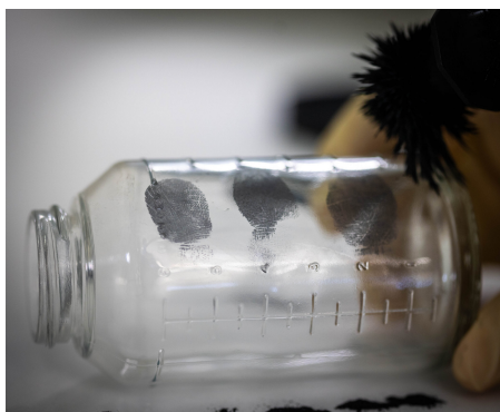
Figure 2: latent prints left on a jar, visualized via charcoal
