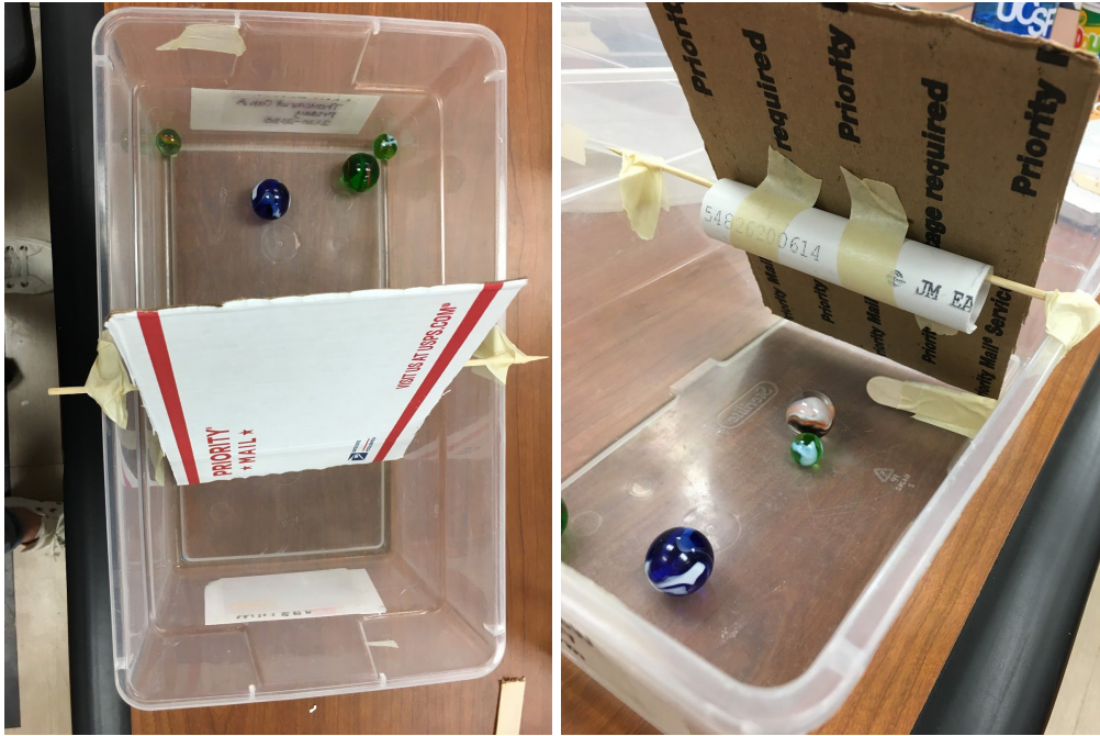
Figure 8a and 8b: Example 1: The piece of cardboard rotates around the axis. A popsicle stick stops the cardboard from rotating in the opposite direction.
