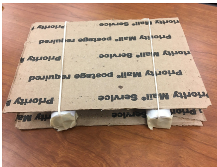
Figure 10: A simple shake table
