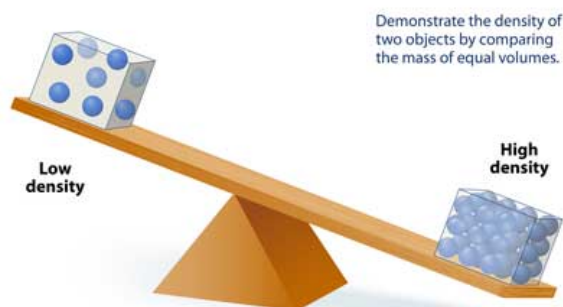
Figure 1: Density Comparison If two objects have the same volume but one has greater mass, the one with greater mass will be considered more dense. LabQMC.
