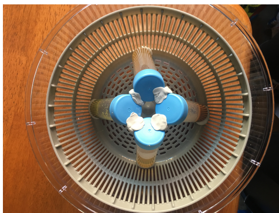
Figure 10: Orientation of tubes in salad spinner. There should be a piece of putty under each tube (sticking it to the spinner) and a piece of putty between the caps of each tube. Stephanie's photo archive.
