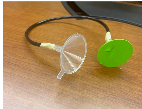
Figure 1: Tape the funnels to the tubing to make the stethoscope
