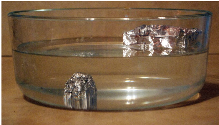
Figure 5: The tin foil ball has more pressure in a single point and less surface area, resulting in it sinking. The tin foil boat has more surface area, reducing pressure at a single point and displacing a greater volume of water allowing it to float.
